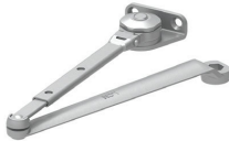
4040XP-3049 Hold Open Arm (H) Non-handed Mounts pull side or top jamb with shallow reveal, hold open adjustable shoe 4040XP closer includes 4040XP-62PA shoe required for parallel arm mounting Optional
